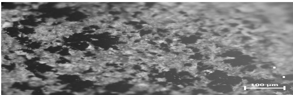
Fig. 3. Microstructure of porous polystyrene C_8H_8 + amorphous colloid Fe(OH)_3 , az adsorption centres of over the norm concentration Mn^{2+} after oxidation of acydofilny microorganisms Fe^{2+} \rightarrow Fe^{3+} after 10 functioning years
