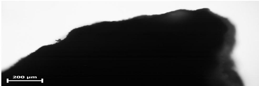
Fig. 2. Microstructure of surface irregularities h = 24 \pm 8 mkm of mineral zeolite Ca[Al_2Si_4O_{12}]x2H_2O before loading into the filter
