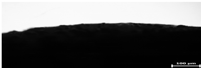
Fig. 2. Microstructure of surface irregularities h \approx 20 \pm 5 mkm C_8H_8 porous polystyrene foam + iron-manganese crust (IMC) - film of higher Mn oxides: pyrolusite MnO_2 , mangosite MnO , Mn_3O_4 , Mn(OH)_2 followed by its oxidation to manganate, MnO_x manganite ( 1 < x < 2 ), todorokite (Mn^{2+}, Ca)Mn^{4+}_3O_7 \cdot nH_2O after 10 functioning years
