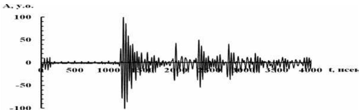
Fig. 4. The window illustration of data treatment of quasilongitudinal elastic waves velocity measuring V = 2485 \pm 30 m/sec in porous polystyrene C_8H_8 by impulse-phase method at frequency f = 1 MGz.
