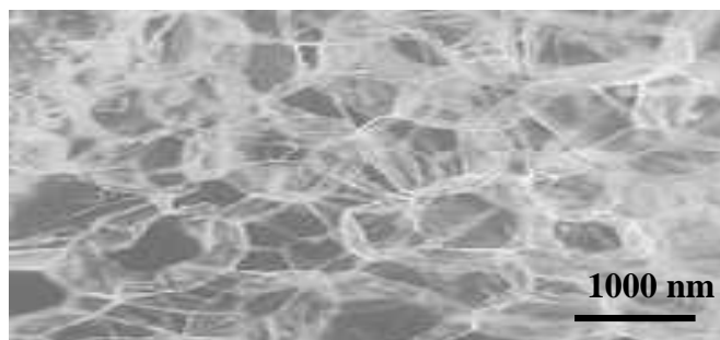
Fig. 1. Microstructure of porous polystyrene before loading at filter.
